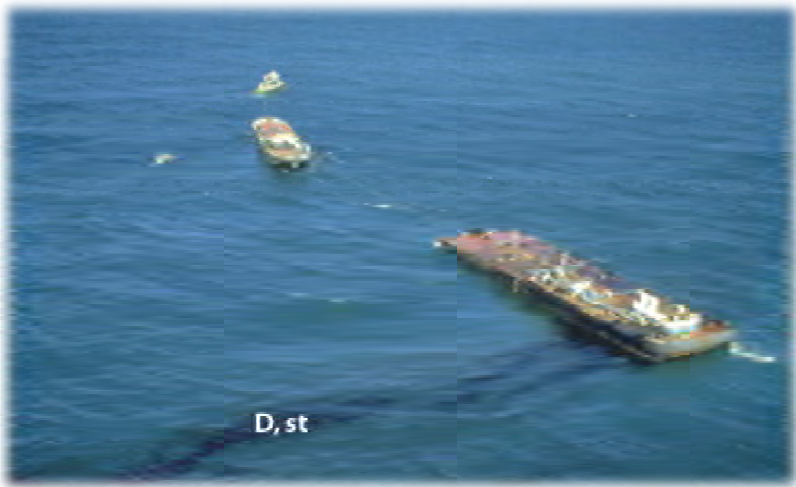
Black Dark (D) Oil - Note the small orange-ish streaks and patches of emulsified oil.
